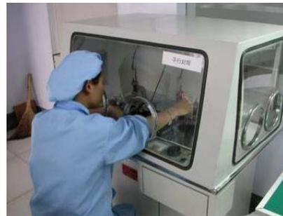
Parallel Seam Sealing Equipment
