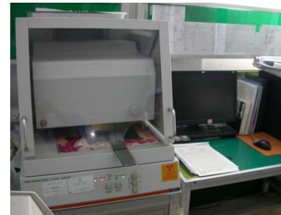
Advanced Plating Thickness Measuring Equipment
